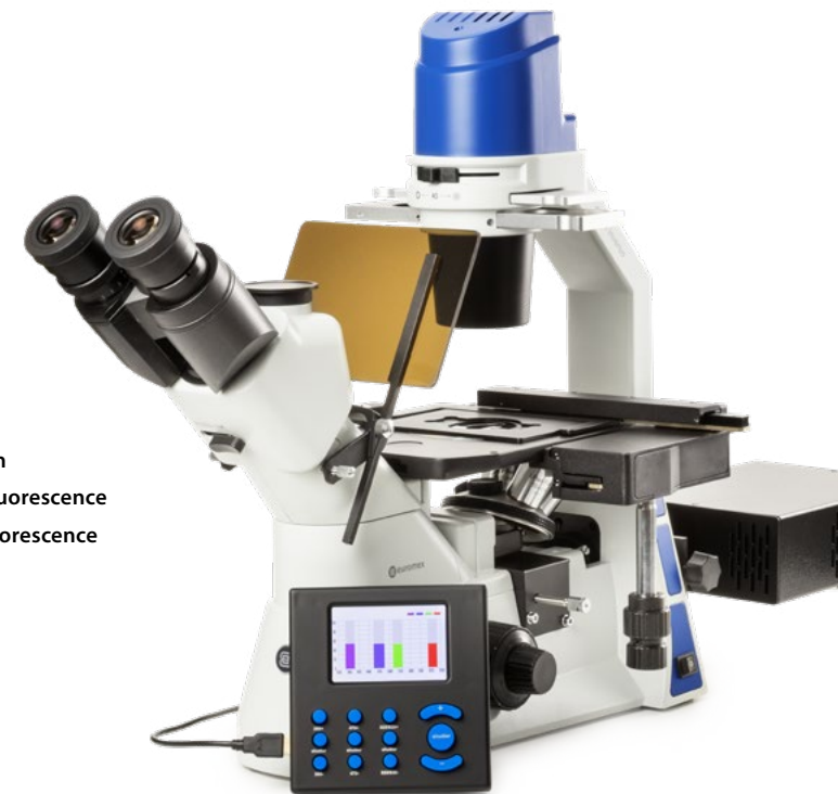
● Oxion Inverso with LED fluorescence (LE.6400)
