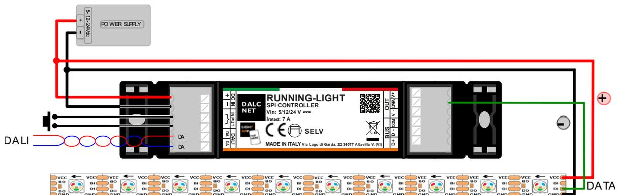
Figure 3: Connection diagram for Digital LED loads (> 7A)
