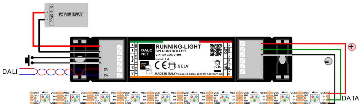
Figure 2: Connection diagram for Digital LED loads
