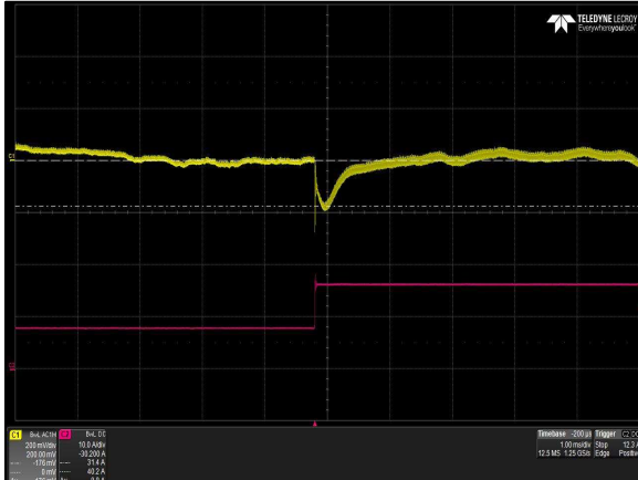
Figure 47: LCC600-36U-9P Transient Response - V_O Deviation 50% to 100% load change 1A/uS slew rate V_{in} = 230V_{ac} Ch 1: V_O Ch 2: I_O
