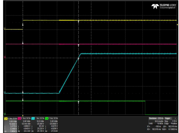
Figure 22: LCC600-28U-9P Turn-on delay via INH_EN
