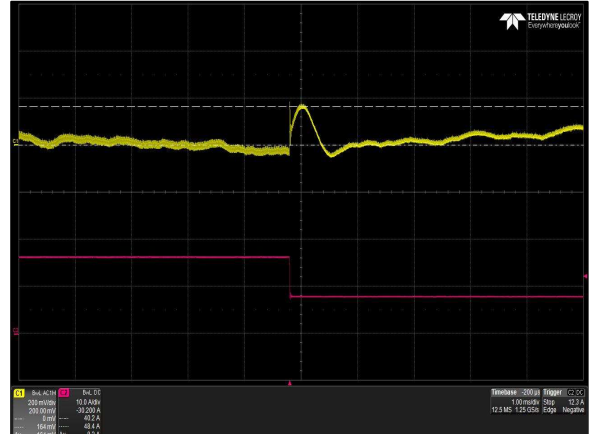
Figure 48: LCC600-36U-9P Transient Response - V_O Deviation 100% to 50% load change 1A/uS slew rate V_{in} = 230V_{ac} Ch 1: V_O Ch 2: I_O
