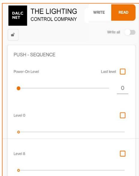
**Power On level:** it is the intensity value to which the output is brought as soon as the device is powered
