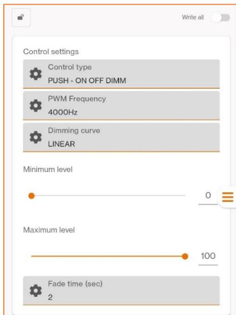
**Control type:** allows you to set the operating logic of the analog input in case of connection to a button or switch.
