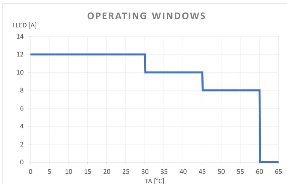
Below are the maximum current values that can be supplied by the MINI-1CV device when the working temperature varies. Ambient temperature [Ta]:
