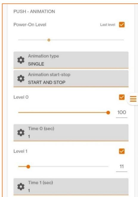
**Power On level:** is the intensity value to which the output is brought as soon as the device is powered
