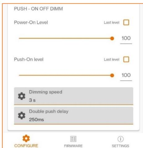
**Power On level:** it is the intensity value to which the output is brought immediately as soon as the device is powered.
