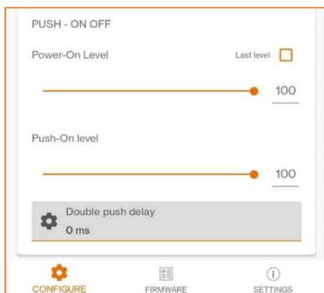
**Power-On level:** it is the intensity value to which the output is brought as soon as the device is powered.
