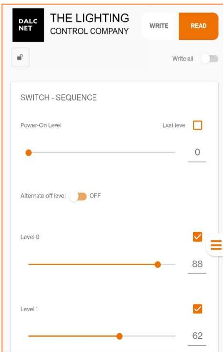
**Power-On level:** it is the intensity value to which the output is brought as soon as the device is powered if the switch is on ON. If the switch is OFF (open) the light will remain off.
