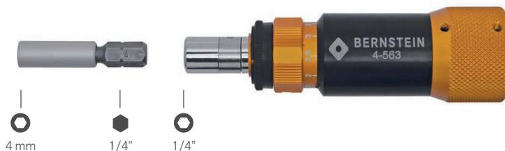
The torque from 0.05 to 0.6 Nm can be set to the required size using a knurled screw, the set value can then be locked. When the set torque is reached there should be an audible click and a click should be felt. If this is not the case, please readjust the small screw so that the screwdriver clicks audibly. When not in use, return the torque-screwdriver back in starting position (0 Nm). This relieves the preload and prevents premature wear.
