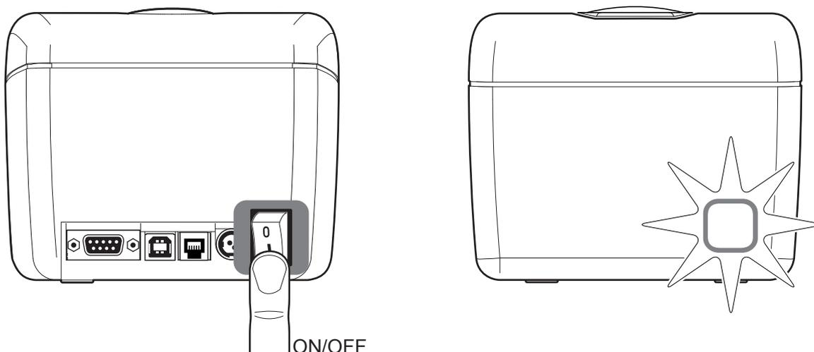
Switch device on pressing key ON/OFF, the LED is switched on and the device is ready.
