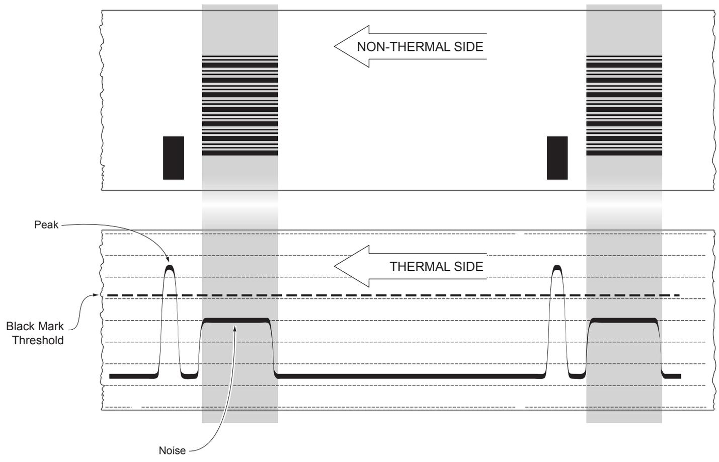
If the maximum value of “noise” read by the sensor is very close to the peak value, it might be difficult to place the value of the “Black Mark Threshold” at an intermediate point. In these cases, it is mandatory that the portion of paper between the point of printing end and the front of black mark is completely white (no graphics). In this way, the only next graphic detected by the sensor for alignment after the printing end will be the black mark.
