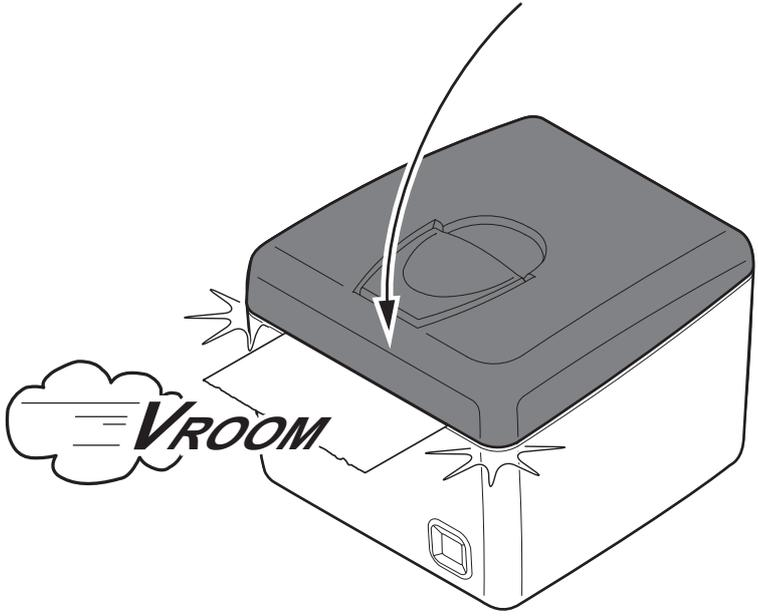
Close the device cover and wait until the paper is automatically loaded .
