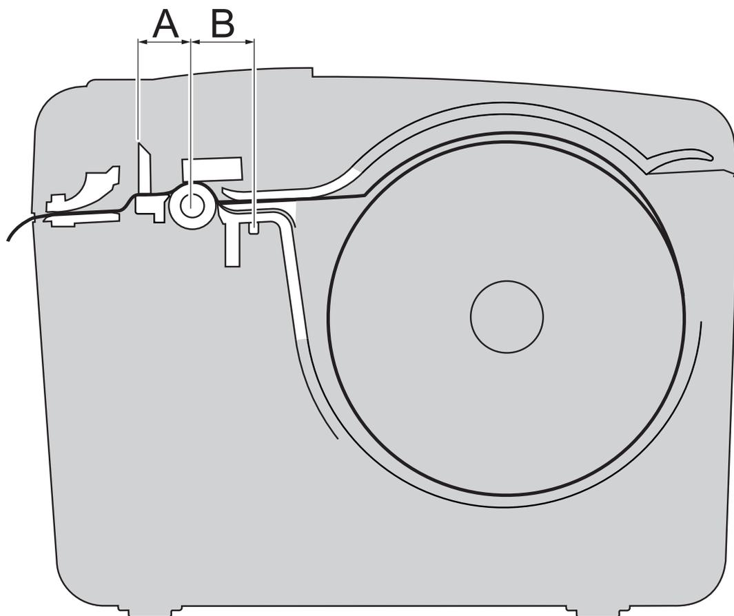
A = distance between printing head and cutter = 13.5 mm
