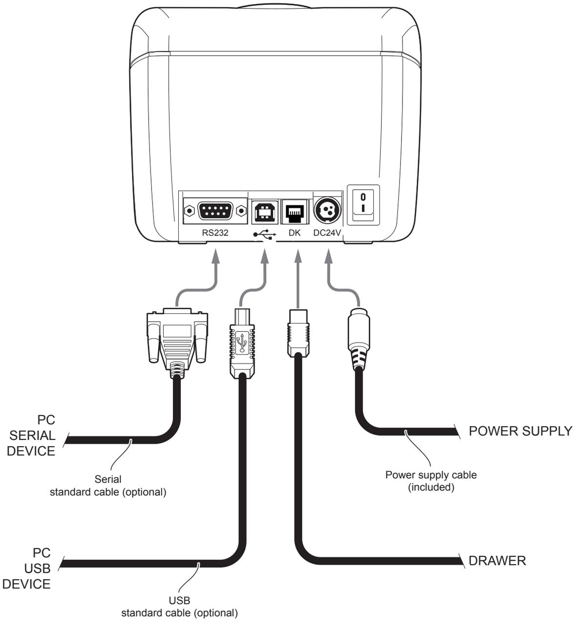
NOTE: When RS232 and USB communication cables are connected to the device simultaneously, the communication takes place via the USB port.
