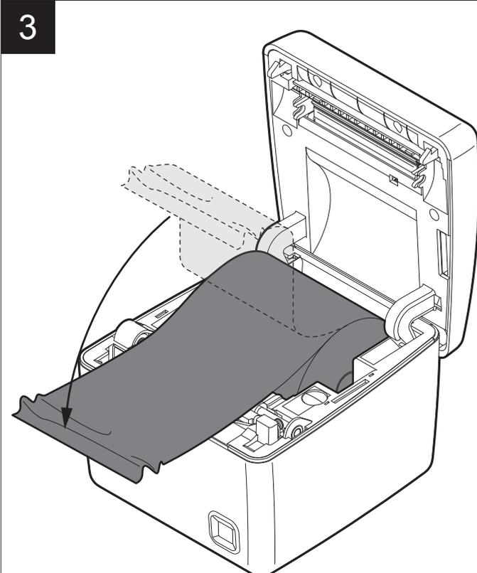
Pull the paper in order to have the damaged part
