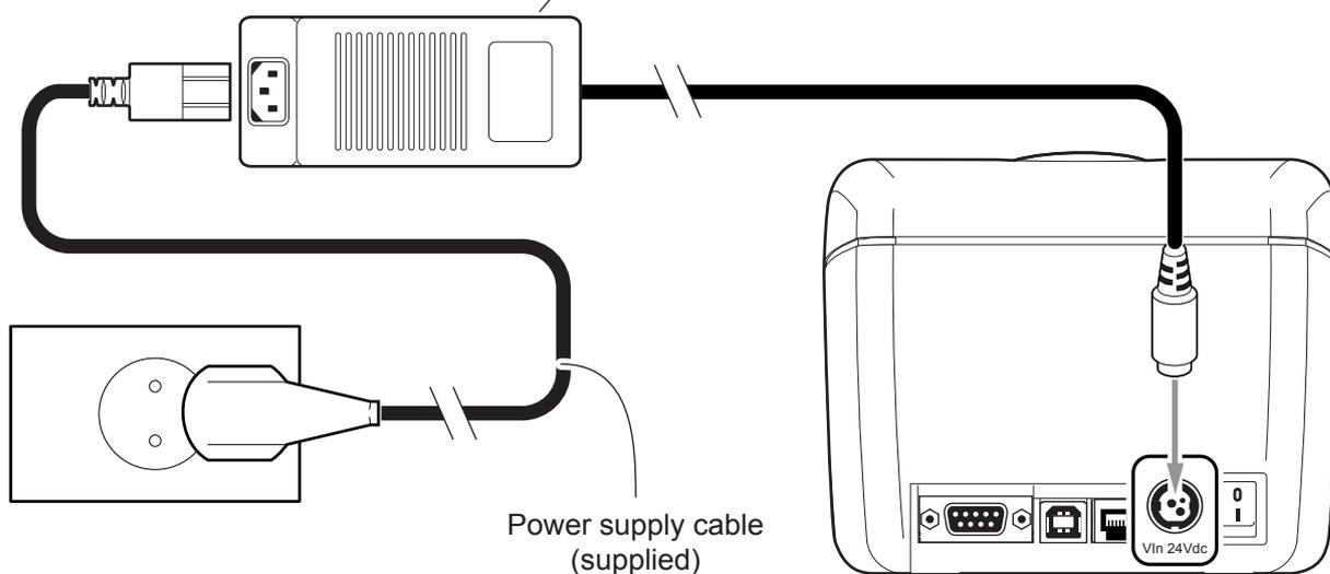
Connect the power adapter (supplied) to the device and the mains outlet.
