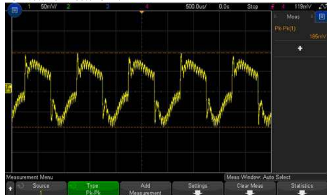
FULL /0% LOAD 50%DUTY / 1KHZ
