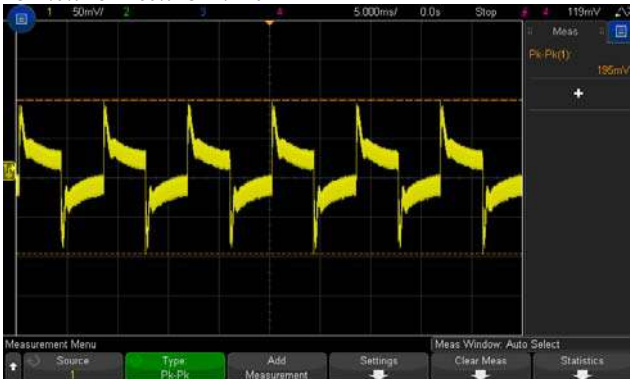
FULL /0% LOAD 50%DUTY / 120HZ
