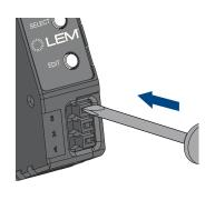
To remove wiring easily, use any tools or a 2.5 mm flat screwdriver
