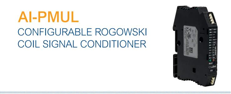
The universal Rogowski coil integrator Al-PMUL complements LEM's flexible clip-around coil ART and ARU range. The design is based on digital processing to give combined dynamic range, accuracy and versatility of use. It offers a wide range of output signals both RMS and instantaneous. AI-PMUL is DIN rail mounted and can be stacked for multiphase application without spacing thanks to its low power dissipation.
